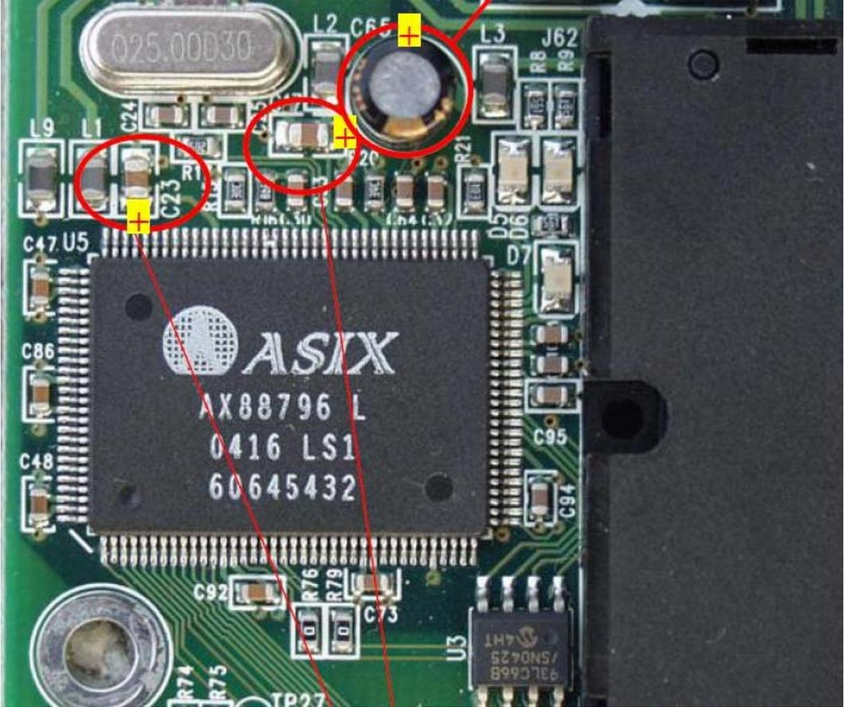
Parallel solder the 4,7uF/16V tantal capacitors on top of these two.
