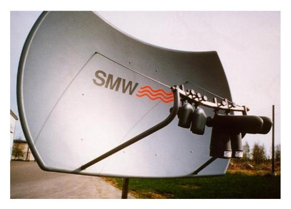
The design is a combination of an offset parabolic and spherical dish, which allows multi satellite reception maintaining a high efficiency for all satellites received.
