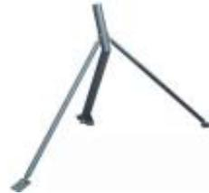
The CHA-WR238P Penetrating mount is a 2-3/8 inch O.D. pipe and is designed to support 90cm through 1.2m antennas onto existing wall structures using appropriate hardware to secure the mount position.
