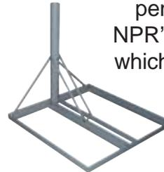
Patriot Non-penetrating mounts are designed to mount antennas onto existing roof structures without penetrating or altering the roof. NPR's are held in place with ballast which varies with antenna elevation and antenna size.
