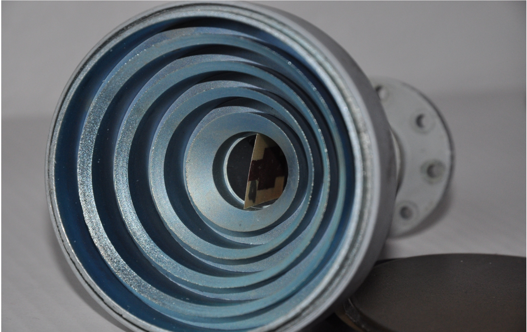
The Delolarising plate, which I used for these tests of circular signal reception from 36E, was a self-made plate (out of a circuit board). This is the best performing plate I've ever
