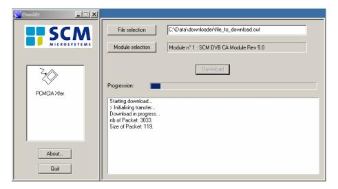
When the download is finished, you should get the message: "Download procedure successful > End of transfer". Now, you can extract your module and insert it in your decoder.
