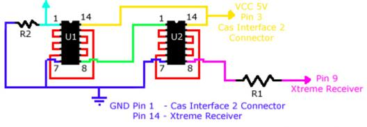
Slow Down Circuit for Xtreme U1,U2 = 74HC04 receivers Only!! U1,U2 = 74HC04 R1 = 100 Ohm R2 = 10K Ohm
