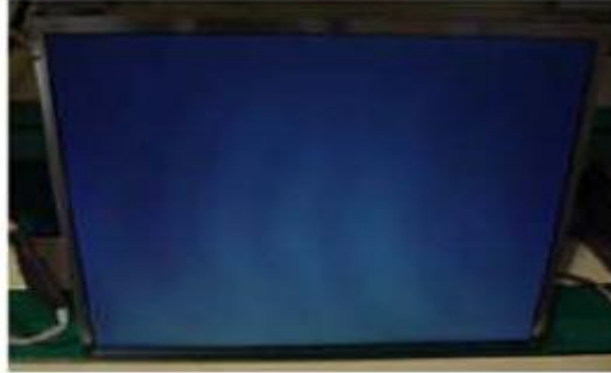
Panel Mura, Light leakage
