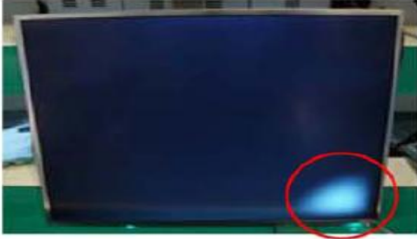
Panel Mura, Light leakage
