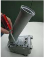
4. Hammer the Screw 1, 2 & 3 slightly via another screw driver or smaller hammer as right picture.
