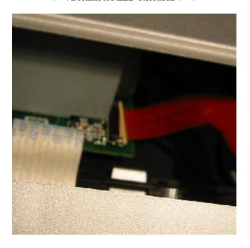
Then Hold the Paper ribbon firmly and pull it out steadily, and try not to bend the pins - don`t worry, it "snaps" back in easily :)
