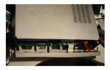
Inside the Dreambox, unclip the Orange ribbon Cable on each side, and slide it out (shown unclipped on one side below)
