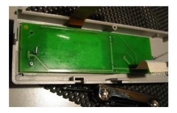
And lift it off.. See the LCD panel below? see the Gap above it? This is where the LEDs poke through and backlight the display.. you MUST re-attach the LEDs so they sit neatly in this gap.. so give it a good look now, and note How far down the board the LEDs are attached.. It's important you put the new ones on in a straight(ish) line to keep the display-light even..
