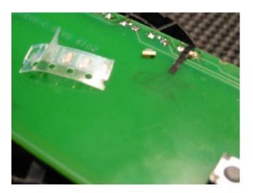
After doing the 6 LEDs, Re-assemble your dreambox and check the light is even accross the display.. if parts are dim, you should be able to work out Which LED needs moving and you
