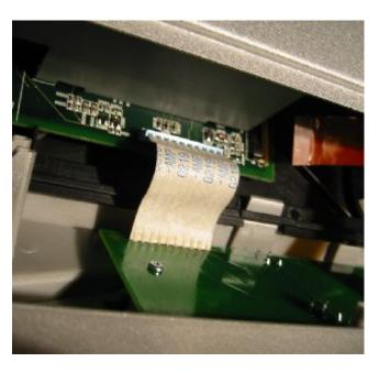
Undo the 3 Small Torx (T20) screws from the LED board..
