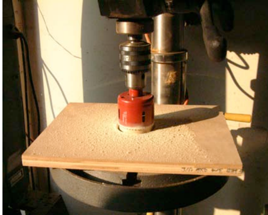
Cutting the hole for the projection lens
