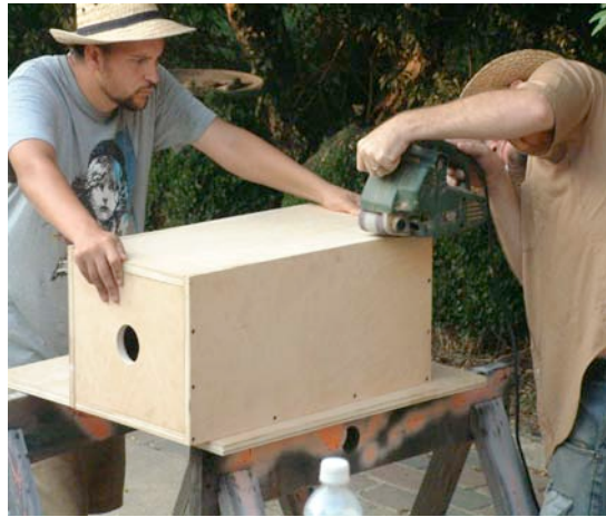
Finishing the prototype enclosure. Note there is no focusing mechanism. I didn't need one for this projector because I knew the distance to my screen and my projection lens has a flange that allows about 1/2" of travel forward and backward for fine focus. If you plan to use your projector in a variety of settings you should make the panel that the projection lens is mounted on movable by about 2 inches.
