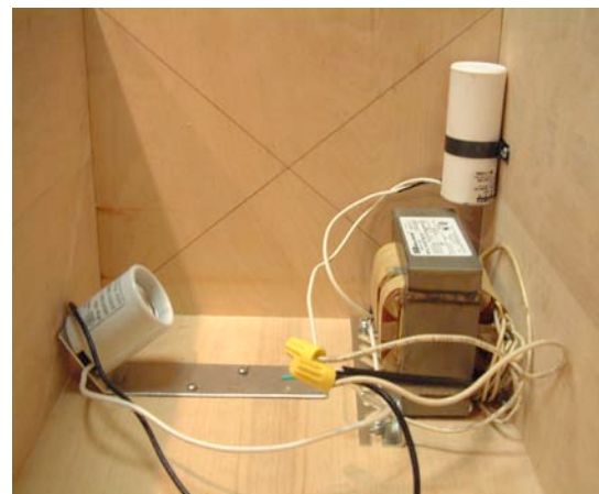
Mounting the ballast, and mogul base. Note the base is mounted at an angle. This is necessary in my enclosure to put the center of the lamp on center with the optics. Note the center reference marks on the back panel.
