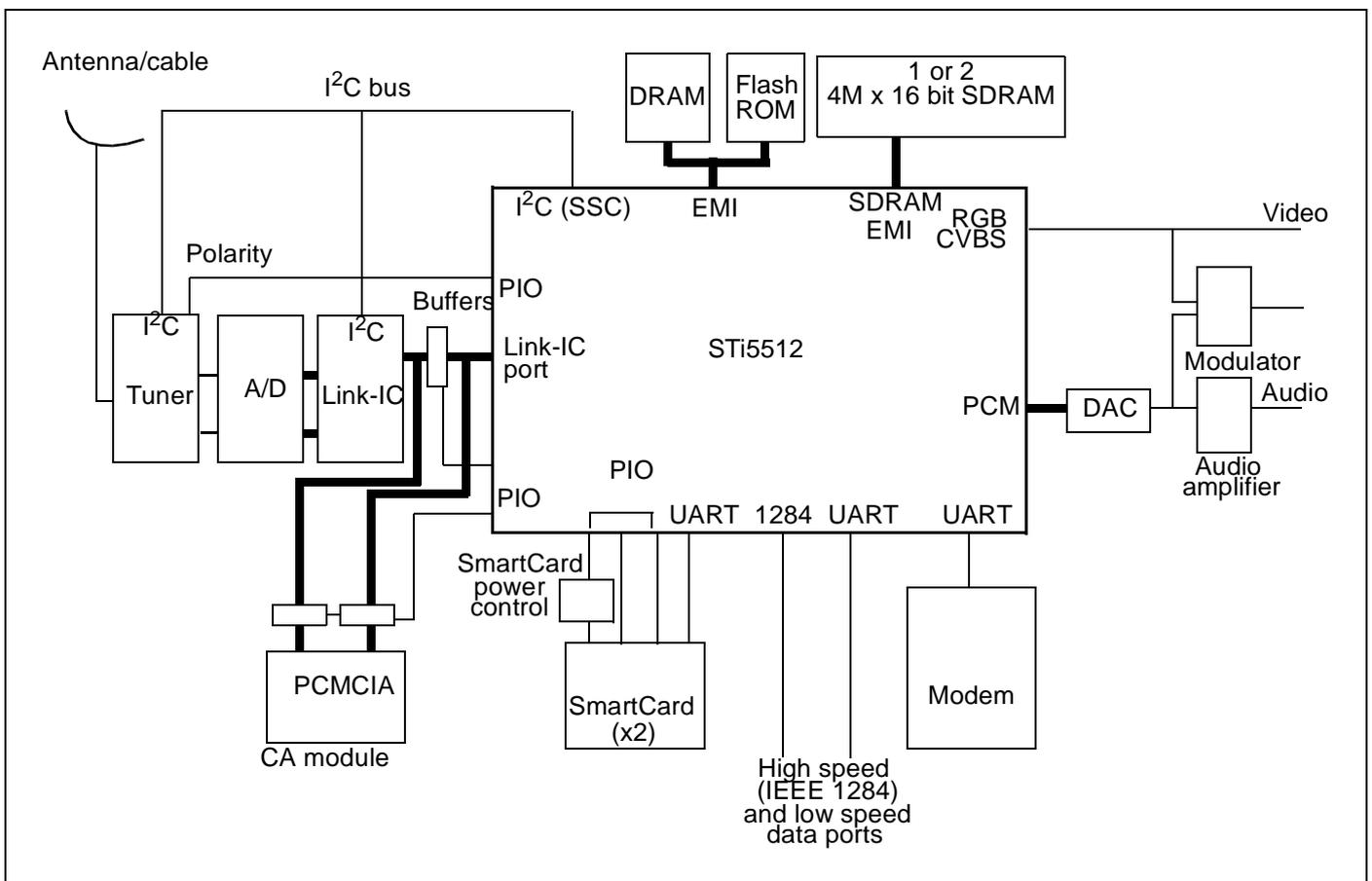
Figure 1 Digital set top box block diagram
