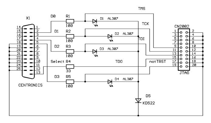
D1, D2, D3 and D4 are 5mm yellow leds. D5 is a 1N4148 or 1N4007 diode. R1, R2, R3 and R5 are 100 ohm resistors. R4 is a 33 ohm resistor
