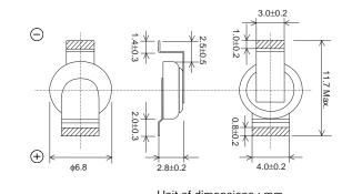
Unit of dimensions : mm Hatched parts are solder plated
