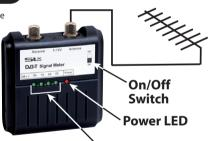
Signal Strength LEDs
