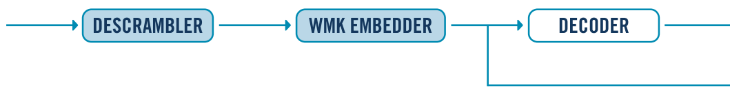
Figure 10 – Replacement model [7] embedding is applicable at descrambler level in a STB
