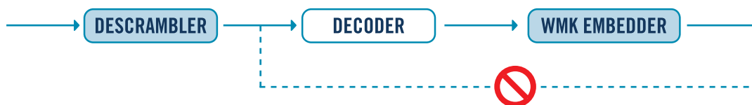
Figure 9 – Conventional watermark embedding at picture level is not applicable to compressed content flows
