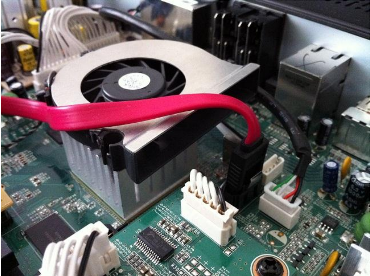
Sadly enough, the SATA cable partially blocks the airflow. Notice that that the cooling fan is connected on the heat sink with just one parker.
