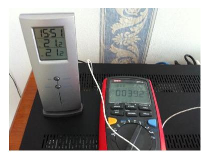
Just a couple of minutes after turning off the fan mounted on the CPU heat sink you can see the temparture rising inside the ET9000. Also notice that the temperature around the ET9000 rose 1 degree in this short time!
