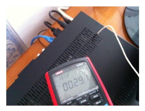
This is the tempature around the tuners and voltage regulators
