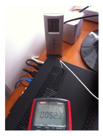
Here the temerature around the voltage regulator, again 1 minute later. These numbers and much higher (Before the mod I mesured 65-72 degrees) where the reason for the modification.
