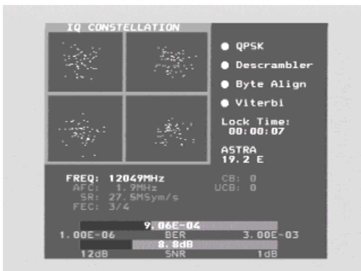
The window also displays the following Digital readout:
