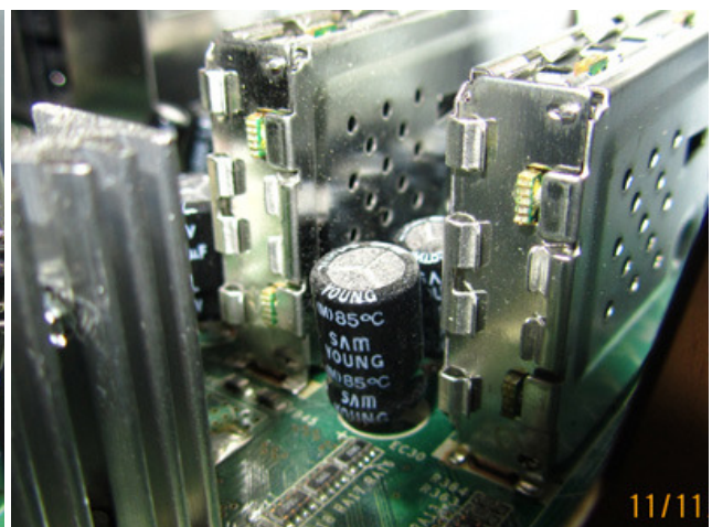
Zooming in on the caps near the tuners (ET9200 - Left | ET9000 -Right)...
